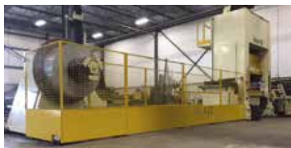
Dilast recently added a feed line with a de-coiler that can handle up to 10,000 pounds. The servo drive feeder can run up to 36.0" wide material.
