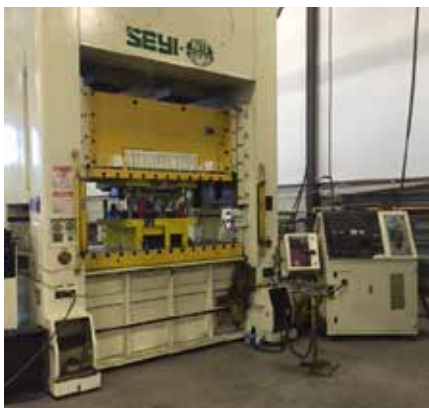
Dilast's newest press addition, a 220-ton SEYI variable speed (0-72 strokes per minute) with full automation capabilities.
