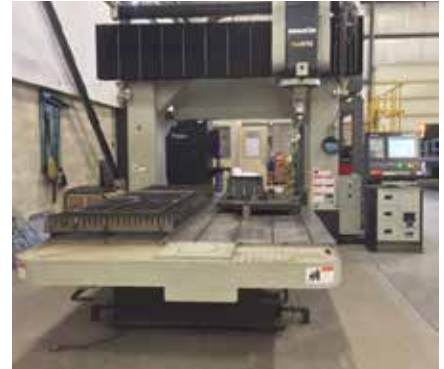
A brand new Komatsu TLM610 5-axis laser cuts costs and time during the die development process.
