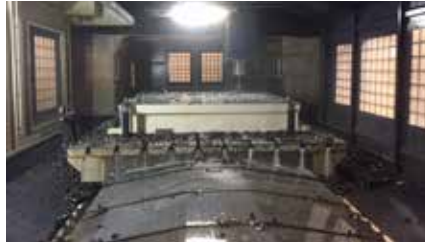
A Takumi H32 bridge type mill with great capacity (77.0 in the Y axis and 126.0 in the X axis).
